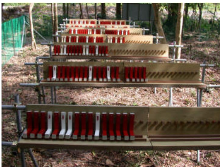
Figure 2. L-joints exposed in Malaysia. Photo: DTI 2005.
