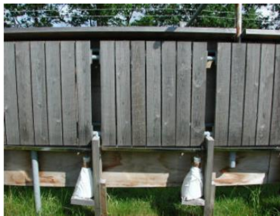
Figure 7. Untreated Scotch pine after 2 years of natural exposure towards south.
