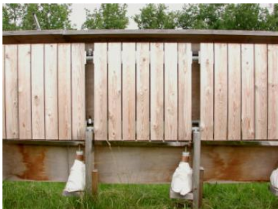
Figure 6. Supercritical treated spruce (SC100) after 2 years of natural exposure towards south.
